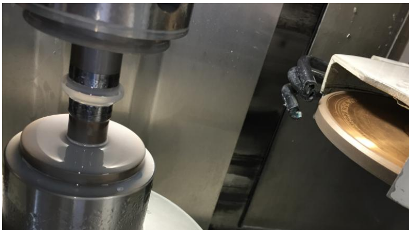
Center grinding a bi-convex lens by bell chucking.
