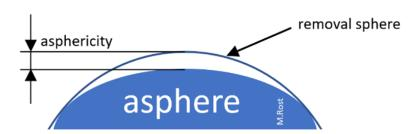
In contrary to optics design, PanDao defines asphericity as the maximum vertical distance from the "removal sphere" to the aspherical, off-axis aspherical or freeform surface.
