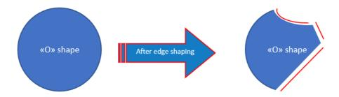
PanDao asks the <u>overall **non-circular circumference** length</u> which is the overall length of the non-cylindrical shapes along the lens perimeter as indicated with the red lines in the example above.
